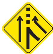
Free flow (added lane)
